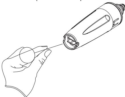
For the adjustable nozzle, you can lubricate the nozzle collar (high pressure to low pressure) by using non-water soluble grease regularly.
