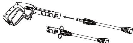
B Insert the spray adjustable nozzle(8) into the extension wand(9),as quick-connect type,you just need push it onto extension wand(9) directly and powerful until hand tight to lock it in place.When the pieces are joined properly, you cannot separate the two components by pulling straight out on the extension wand(9) .Insert the Turbo nozzle in the same manner, depending upon which attachment is best suited to the surface you are cleaning.Only one attachment can be inserted into the.
